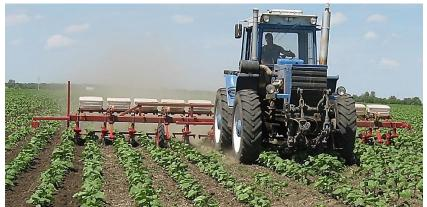
Fig. 2. HTZ-16131 tractor with KRNV-8.4 cultivator
